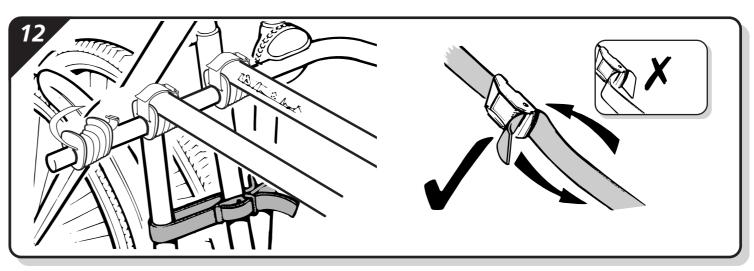
When carrying a second or third cycle, feed the RED straps around all in the cycles falling off the carrier. To reduce obstruction from the cycles frames, and fully tighten. Failure to use these straps will result handlebars, alternate the direction of each cycle during loading.
